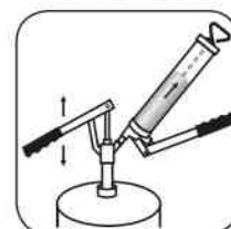
Loading with filler pump (Use 128 003 valve)
