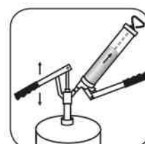
Loading with filler pump (Use 128 003 valve)
